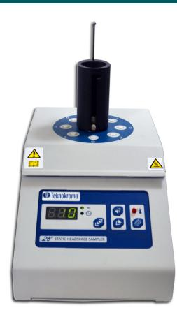
The Manual Headspace Sampler allows users to perform accurate, quantitative, and repeatable static headspace analysis without the need for an expensive autosampler. The sampler can incubate up to 6 sample vials at a time, whilst also ensuring the syringe is heated to the same temperature. Adjustable timers with alarms for sampling and equilibrating times make operation simple and easy to use.
